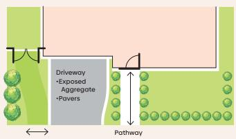
Secondary Driveway to be constructed of gravel, lawn or other permeable material
